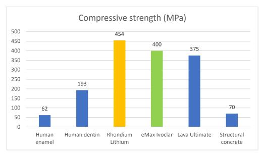
Figure 1. Compressive strength comparison with other CAD/CAM materials
