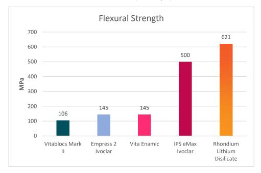
Figure 3. Flexure strength of ceramics comparison graph
