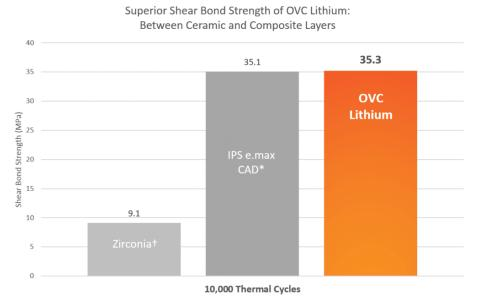
Figure 11. Bond strength of lithium layer to composite sub-layer
