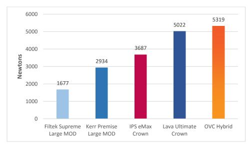
Figure 6. Fracture resistance graph - average maximum load at failure
