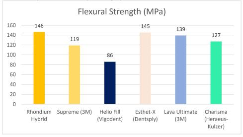
Figure 4. Flexure strength of composite comparison graph
