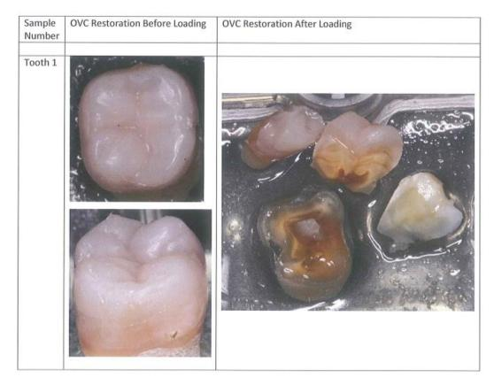
Figure 7. Typical example of OVC Hybrid crown at maximum load
